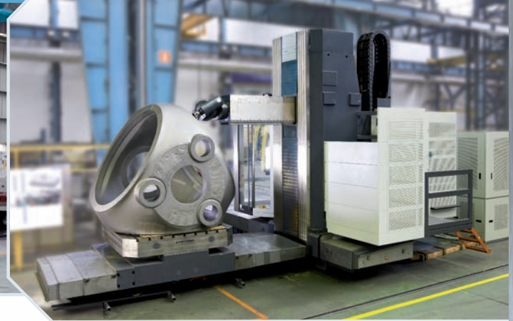
MACHINING OF A WIND TURBINE HUB
