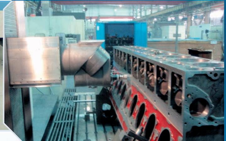
MACHINING OF A MOTOR BLOCK
