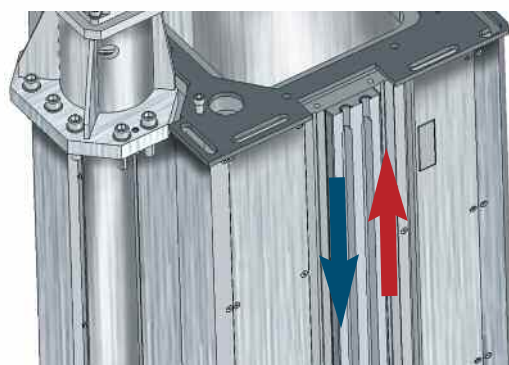
- Cooled friction guide in the ram.
