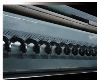
Automatic chip removal (Screw type chip conveyor)
