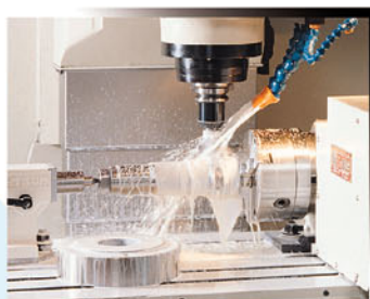
High pressure coolant (P:3.5 kg/cm 2 , Q:100 l/min)
