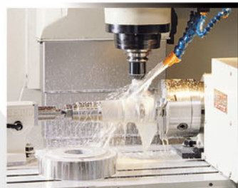
High pressure coolant (P:3.5 kg/cm 2 , Q:100 #/min)
